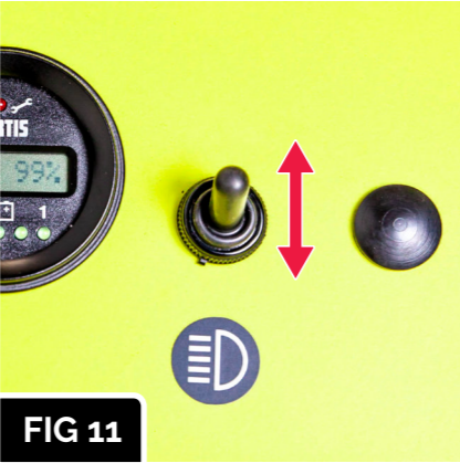
FIG 11 Ensure the light switch is working correctly. If applicable check remote control switch.
