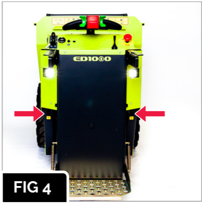
The anchor points location on each lower side at the rear of the truck.
