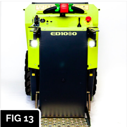
FIG 13 Ensure rear facing lights are functioning and free from debris.
