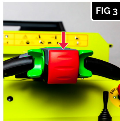
EMR Reverse Protection Switch: When ACTIVATED, will STOP the truck and move forward.
