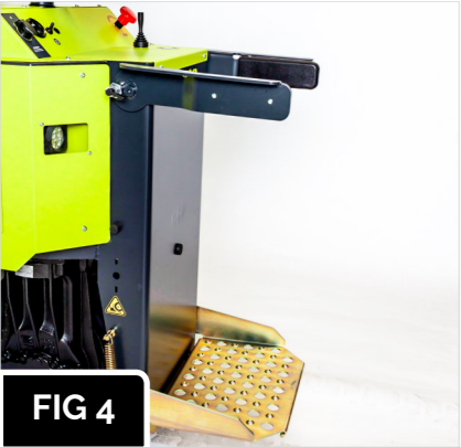
The safety rail locked in the raised position.
