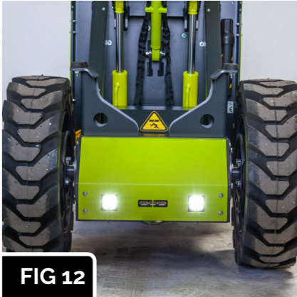
FIG 12 Ensure front facing lights are functioning and free from debris.
