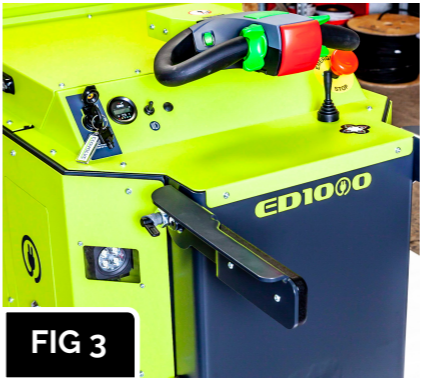
FIG 3 The safety rail locked in the raised position.
