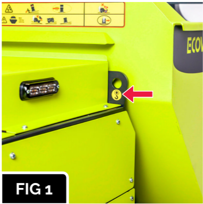
The lifting point locations are identified by this symbol.
