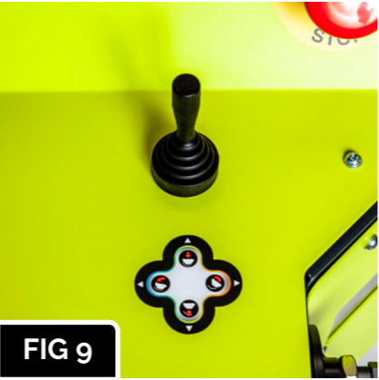
FIG 9 Skip lever. Ensure all 4 functions work correctly.
