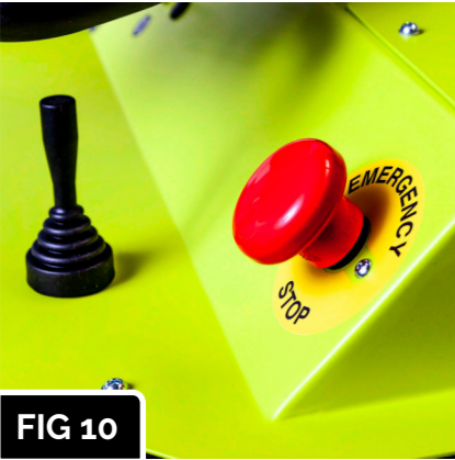
FIG 10 Check the emergency Stop button. When pressed in shuts machine down.
