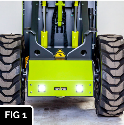
FIG 1 Inspect the front and rear wheels and tyres for wear and damage. Remove any debris if present
