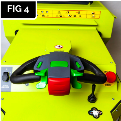
FIG 4 Move the tiller head left and right to check the steering controls.
