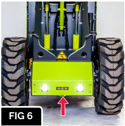
The anchor points locations at the front of the vehicle.
